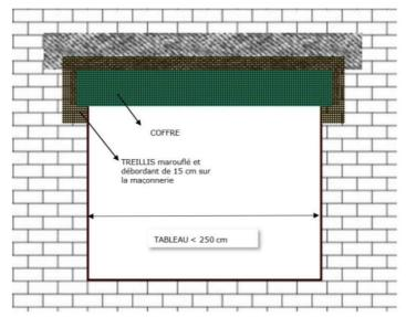
Figure 2 Table < 250 cm: installation of the facade coating with mesh
