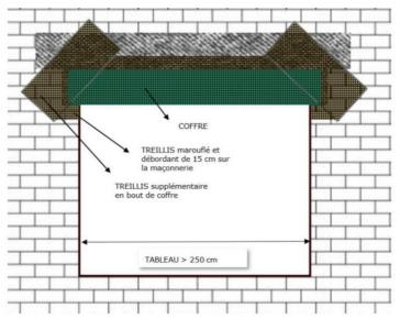
Figure 3 Table > 250 cm: installation of the facade coating with reinforced mesh
