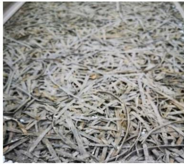
Figure 6 - Wood-cement fiber finish
